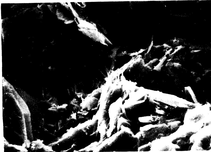
Figure 5. Photomicrograph of freeze dried core sample from 3,530 feet, showing well developed fibrous illites (2,400 X). Long dimension of photo is 50 microns.
