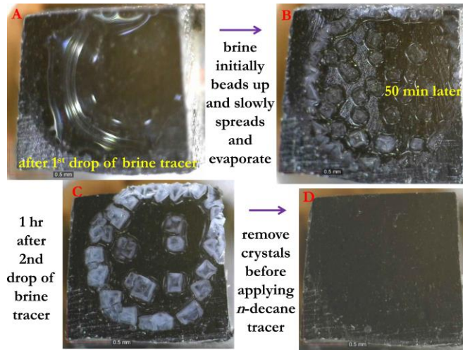
Figure 2. Spreading behavior of traced-API brine on an Eagle Ford sample (a scale bar is shown on each picture).
