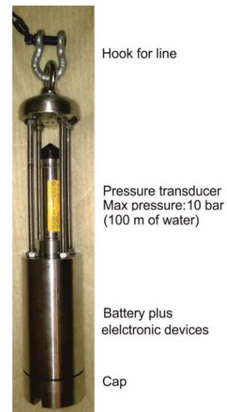
Figure 4: Pressure gauge developed by INiG-PIB
