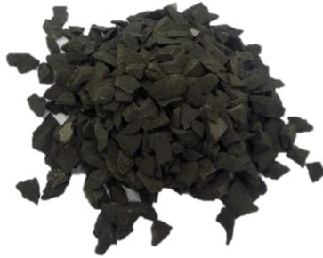
Figure 1. Disintegrated sample of Bazhenov shale.
