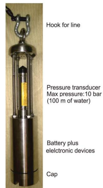
Figure 4: Pressure gauge developed by INiG-PIB
