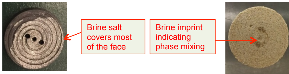
Figure 7: Pictures taken after the test for, (a) face of Elastomer spiral inlet end-piece, and (b) face of the core at the inlet side
