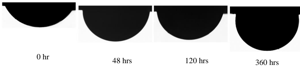
Figure 6: Contact angle of synthetic SW-3S-6C-M at different time intervals of 0, 48, 120, 360 hrs.
